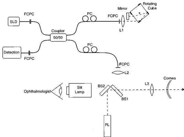
**Fig. 1** Schematic diagram of the experimental setup. SLD: Superluminescent diode; FCPC: FCPC connector; PC: Polarization controller; L1, L2, L3: Lenses; BS1, BS2: Beam splitters; FL: Fixation laser.
