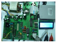
Figure 1. Intelligent DC micro-ohmmeter.
