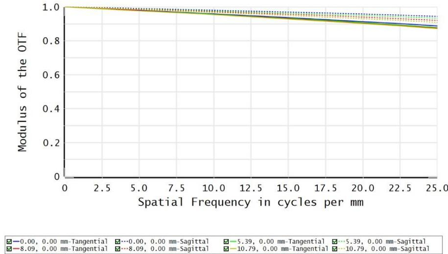
Figure 7. MTF plot for the central wavelength (650 nm) considering pixel size of 20  $\mu\text{m}$  (Nyquist frequency 25 cycles/mm)
