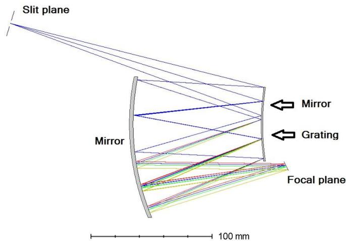
Figure 6. Spectrometer layout
