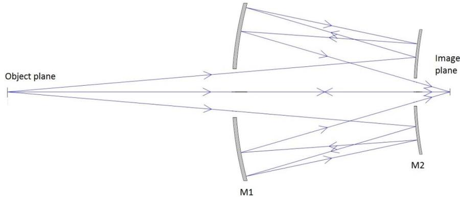
Figure 5. Flat image anastigmat relay
