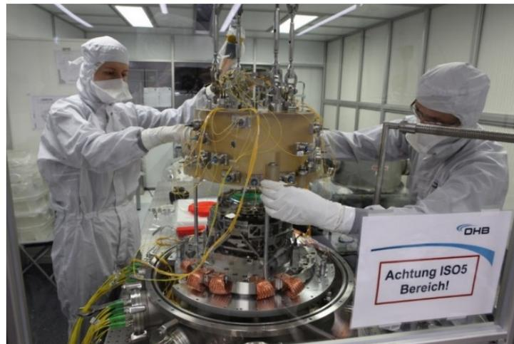
Figure 4-1 CaLA cryogenic alignment test. The ZERODUR structure holds all interferometric fiber optic distance sensors, which monitor the movement of each lens assembly in lateral and axial direction during the thermal cycling
