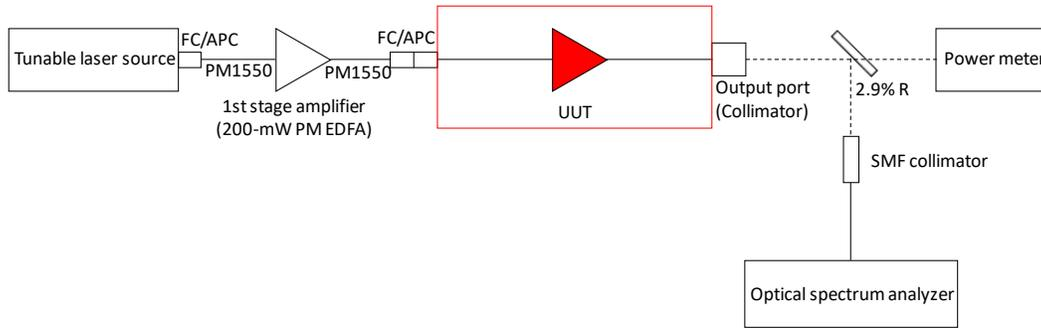
Fig. 3. Block diagram of experimental evaluation for the DP-DC-EYDFA.
