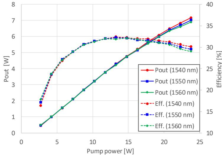
Fig. 6. Measured output power ( $P_{out}$ ) and optical-to-optical conversion efficiency (Efficiency) of the fabricated DP-DC-EYDFA (Wavelength of input signal: 1540, 1550, and 1560 nm, EYDF length: 5.5 m).
