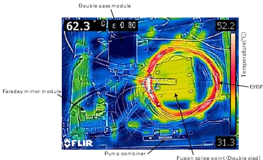
Fig. 9. Measured temperature of the fabricated DP-DC-EYDFA during amplification operation (Wavelength of signal: 1560 nm, Pumping power: 7.2 W, EYDF length: 5.5 m).
