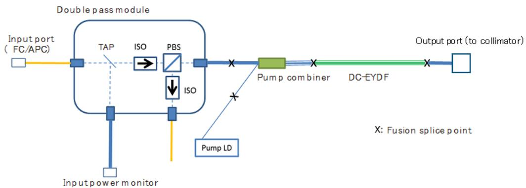
Fig. 5. Block diagram of the DC-EYDFA for SP evaluation.
