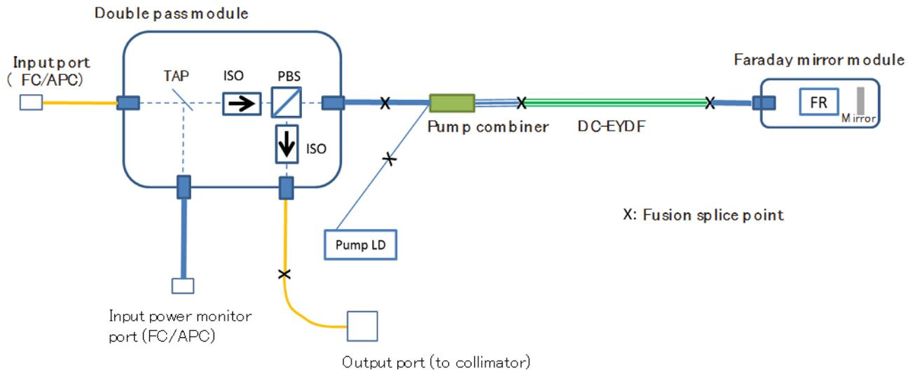
Fig. 1. Block diagram of the DP-DC-EYDFA.
