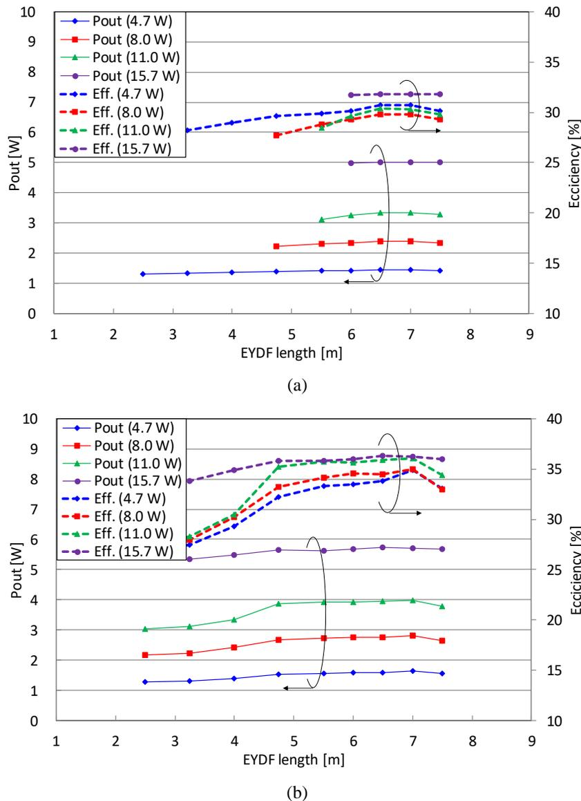
Fig. 8. Comparison of output power (Pout) and optical-to-optical conversion efficiency (Efficiency) between (a) SP operation and (b) DP operation (Wavelength of input signal: 1560 nm, Pumping power: 4.7, 8.0, 11.0, and 15.7 W).
