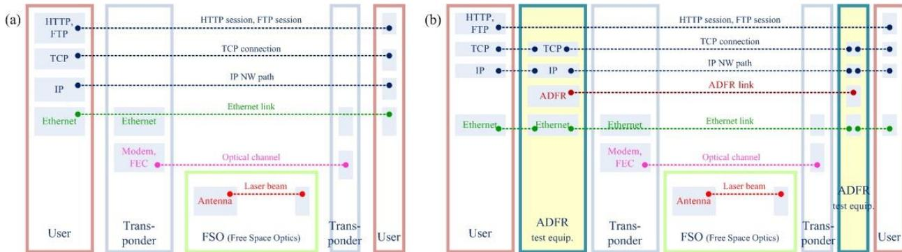
Figure 1. (a) Protocol stacks of the normal FSO communication systems, (b) Protocol stacks of the FSO systems with ADFR (test equipment) explained in 2.3. ADFR test equipment is designed to be inserted between User and Transponder as a simple add-on, and not to influence any versatility of them.
