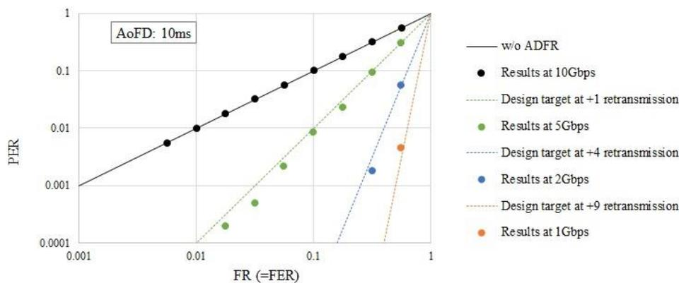
Figure 4. Measured results of the capabilities of PER improvements by ADFR. Due to the statistical characteristics of the fade patterns shown in fig.3 (b), one more additional retransmission makes PER to be reduced accordingly to the raw FER if the retransmission interval was properly selected.
