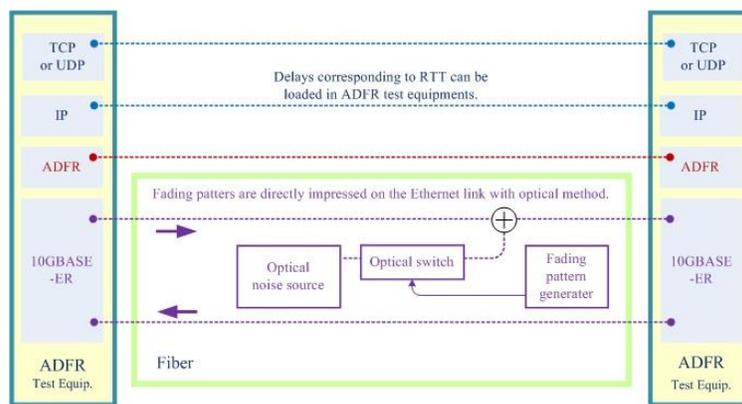
Figure 2. Experimental setup used in the evaluations of PER reduction with UDP traffics and throughputs of TCP traffics. Delay elements to emulate long RTTs are not described in this figure. Fade was generated by adding modulated optical noise on one direction of the signal light between 10GBASE-ER. This low-cost approach however enabled very precise transcription of the varieties of the fade patterns on the signal streams.
