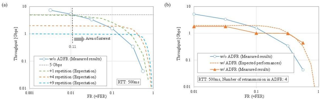
Figure 5. (a) Measured results of the throughput with TCP only, and expected performances with ADFR. (b) Examples of measured results of TCP throughput with ADFR (number of retransmission: 4).
