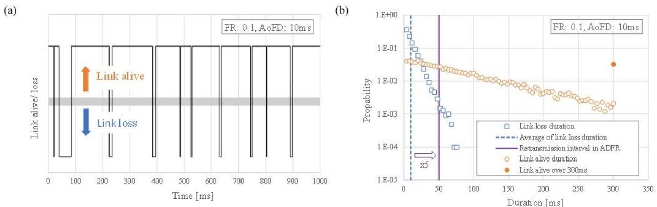
Figure 3. (a) Part of the fade pattern generated with random number generator. Fade ratio (FR) is 0.1 and average of fade duration (AoFD) is 10ms. (b) Statistical properties of the fade pattern in terms of durations of link alive/loss.
