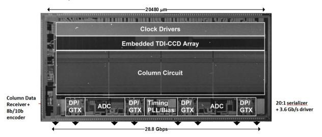
Figure 3 Die design prototype
