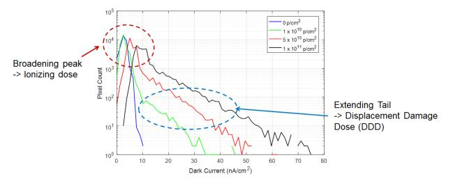
Figure 10 Bright pixel post proton and 14 days room temperature anneal.
