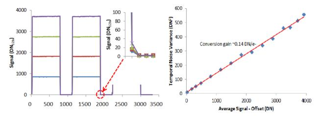
Figure 7 Left CTE measurements and right Photon Transfer Curve.
