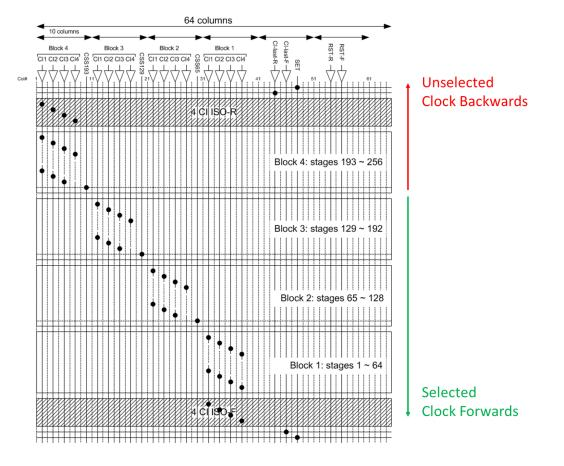
Figure 6 CCD structure phase clocking.
