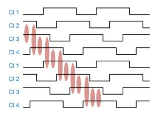
Figure 2: CCD structure phase clocking.
