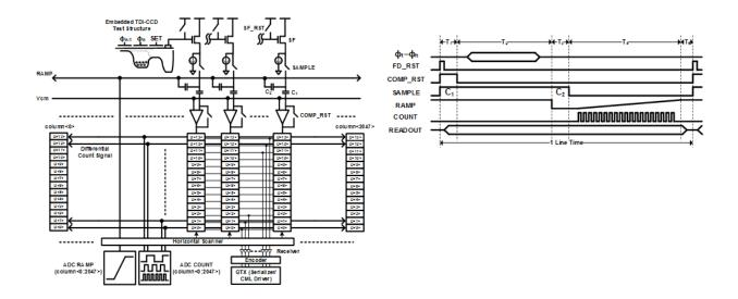
Figure 5 High speed ADC readout diagram and timing.
