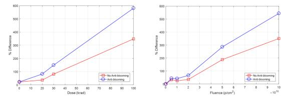
Figure 9 Post radiation dark current: Left is post Gamma and 7 days room temperature anneal; right is post Proton and 14 days room temperature anneal.
