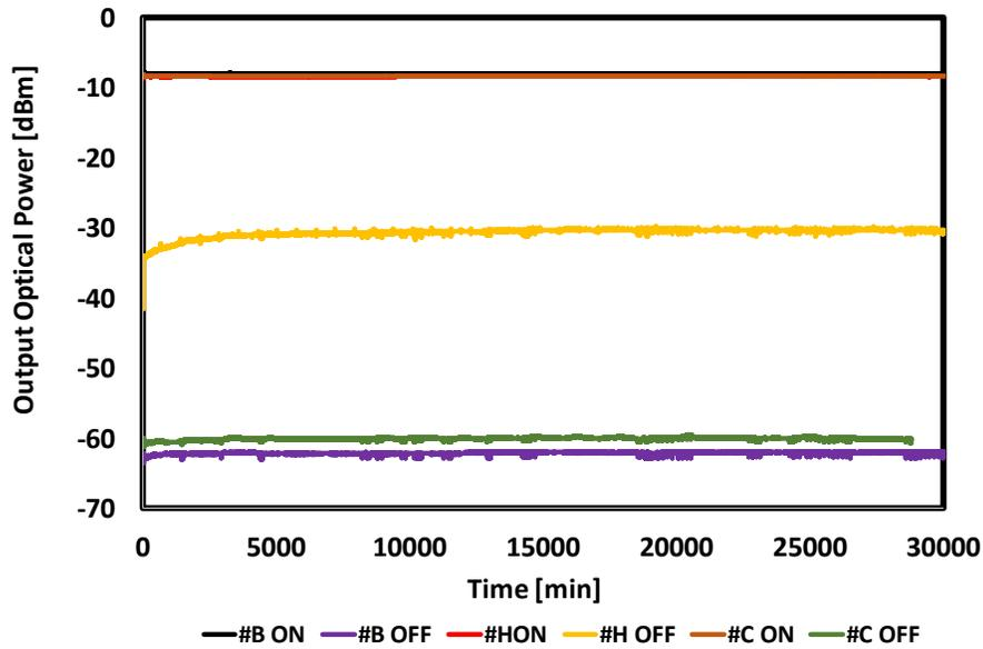
Fig. 3: Measured optical power of several samples during radiation test.
