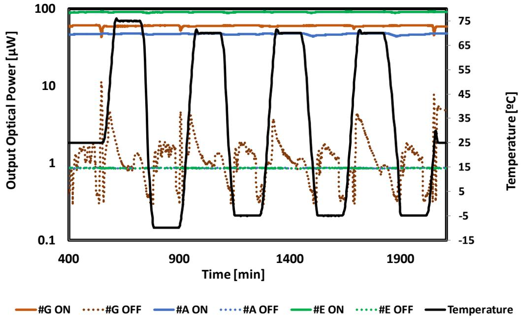
Fig. 2: Measured optical power of several samples during vacuum thermal cycles, and temperature profile.
