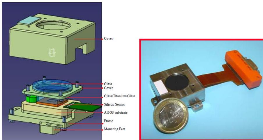
Figure 5: Galileo mini-DSS [3]
