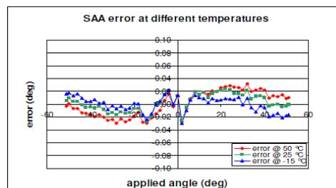
Figure 3: measured errors on prototype mini-DSS [2]
