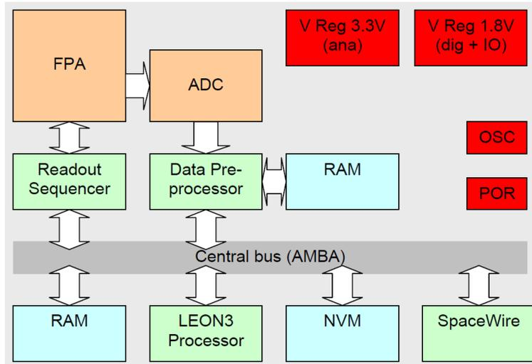
Figure 4: Intended functionality of the LCMS chip [3]
