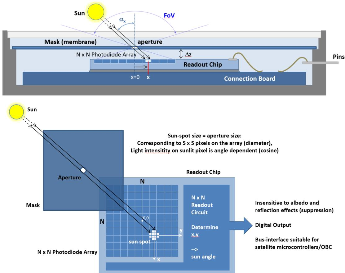
Figure 7: Illustration of the digital sensor chip applied in the IBIS sensor.
