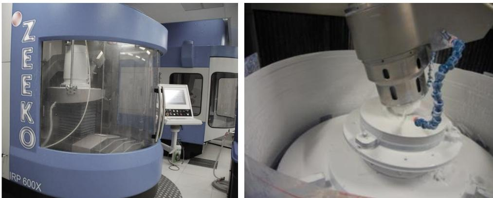
Figure 4. ZEEKO IRP 600X (left, foreground) and IRP 1200X (left, background) installed in Media Lario and example of off-axis aspheric Al/NiP mirror in figuring and polishing process (right).
