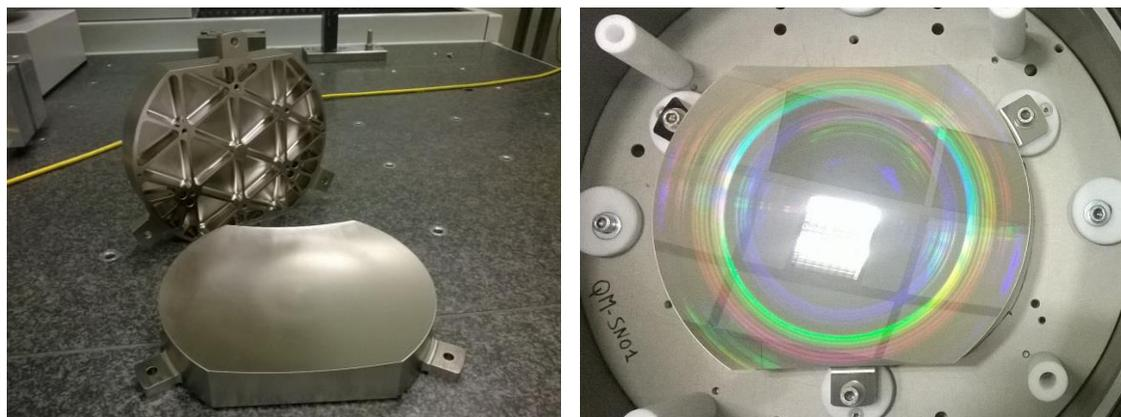
Figure 3. Two HRM mirror blanks after NiP coating (left) and one in the transportation container after final diamond machining (right).
