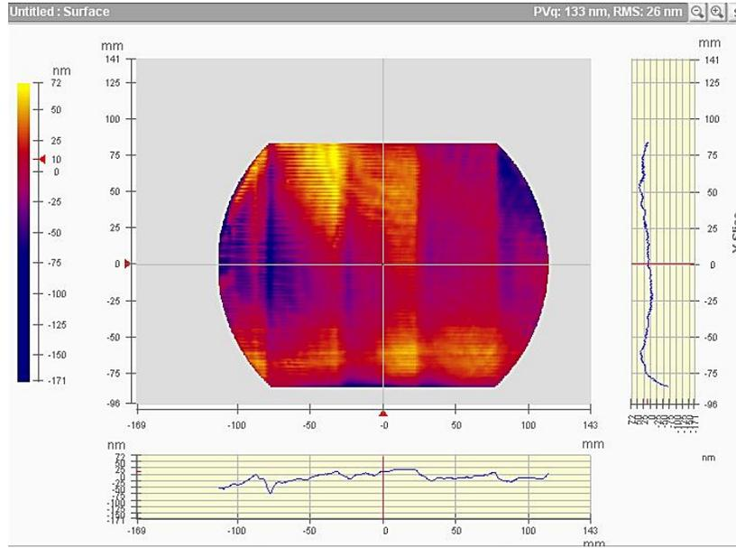
Figure 6. Surface shape accuracy of 133 nm PV achieved on the HR Mirror Breadboard, corresponding to a wave front error of 048 fringes PV.
