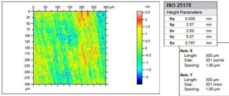
Figure 7. WLI surface roughness measurement of the HR Mirror Breadboard after iterative figuring and polishing on Media Lario's ZEEKO IRP 1200X.
