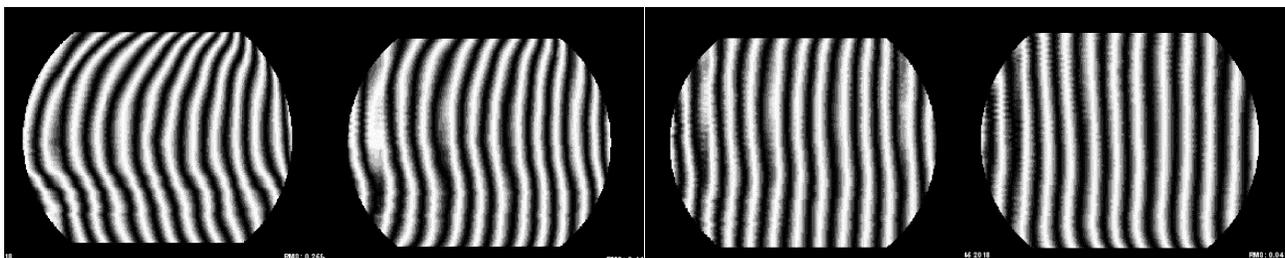
Figure 5. Evolution of the surface accuracy of the HR Mirror Breadboard during the IRP figuring and polishing runs.
