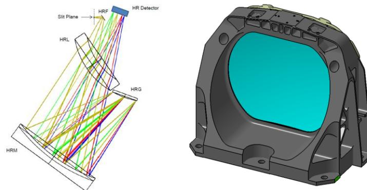
Figure 1. Optical layout of the FLORIS high-resolution spectrometer showing the HRM mirror (left) and view of the opto-mechanical assembly of the HRM mirror (right).
