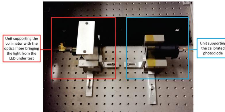
Figure 8. Setup for the calibration of the LEDs.
