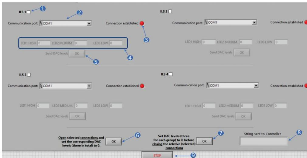
Figure 7. GUI to command the ILS LEDs.
