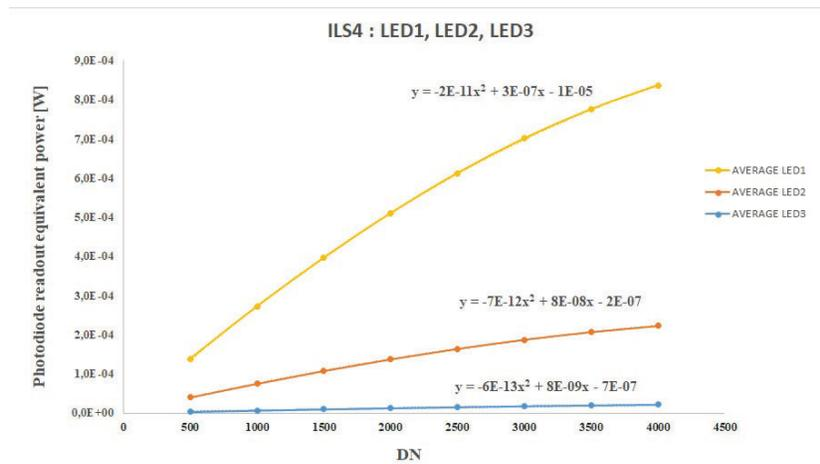
Figure 10. Typical calibration curve of the LED sources.
