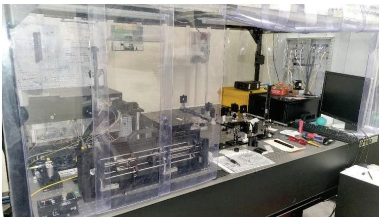
Figure 18. ALASCA optical bench under integration and testing
