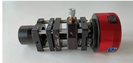
Figure 8. Photo of prototype SHIMM instrument after assembly in the laboratory
