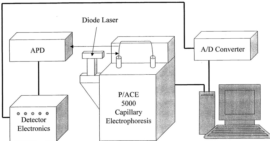
Figure 2 Diagram of modified capillary electrophoresis
