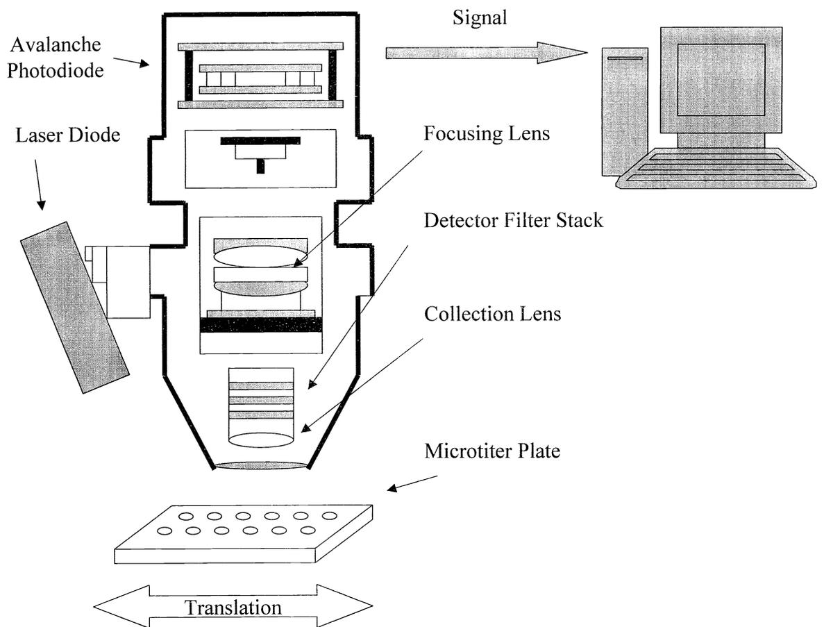
Figure 7 Diagram of near infrared fluorescence immunoassay instrument
