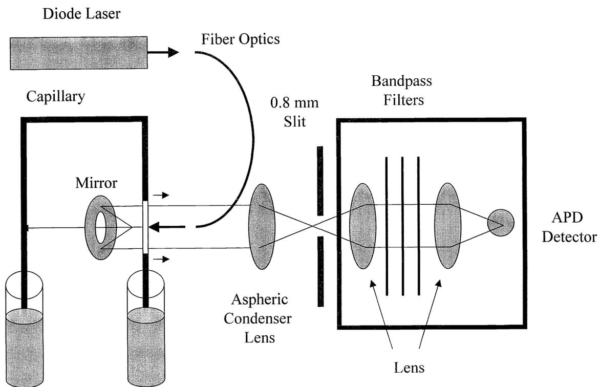
Figure 3 Optical path of capillary electrophoresis
