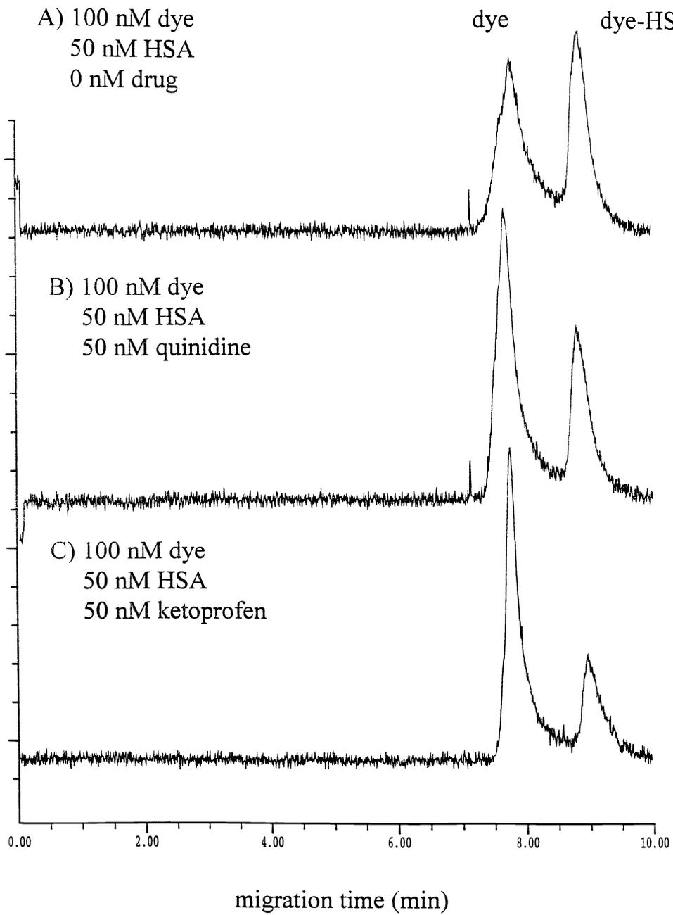
Figure 6 Electropherogram illustrating competitive interaction between drug and dye
