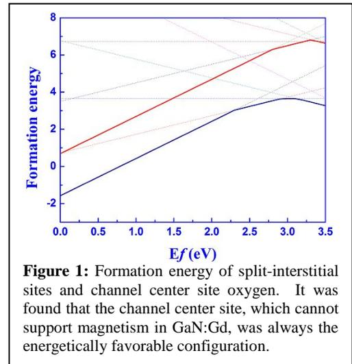
**Figure 1:** Formation energy of split-interstitial sites and channel center site oxygen. It was found that the channel center site, which cannot support magnetism in GaN:Gd, was always the energetically favorable configuration.
