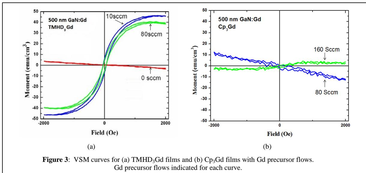
**Figure 3:** VSM curves for (a)  $\text{TMHD}_3\text{Gd}$  films and (b)  $\text{Cp}_3\text{Gd}$  films with Gd precursor flows. Gd precursor flows indicated for each curve.
