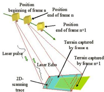
Figure 14 – Lidar assisted autonomous landing
