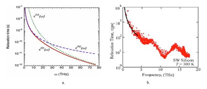
Figure 2. Frequency-related phonon relaxation time in bandgap material [11]: a. calculations, where normal (dashed curve), wide-angle (dotted curve), and total (solid curve) relaxation times plotted as a function of frequency for Si at T=300 K.; b. experiment.
