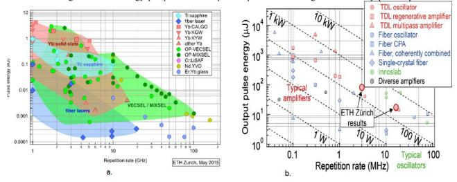
Figure 3. Ultrafast lasers available for pumping. a. nJ per pulse in multi-GHz pulse repetition rate [12]; b. µJ per pulse in multi-MHz pulse repetition rate [13].
