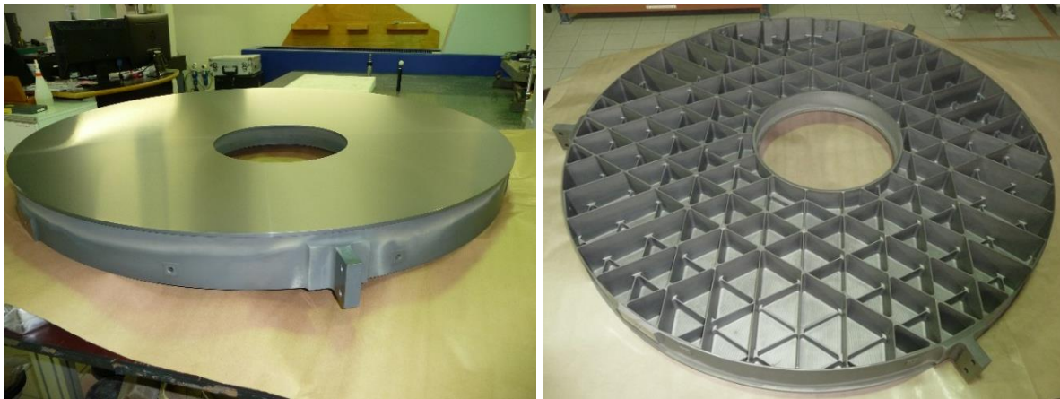
Fig. 7. The ready-to-polish M1 blank Flight Model, front face (left picture) and rear face (right)
