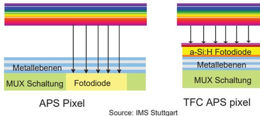
Figure 2 State of the art pixel cell technologies of APS detectors
