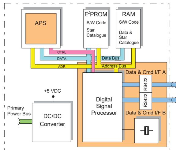
Figure 4 Block diagram for an APS based star tracker reduced to the absolute minimum extend of functional blocks
