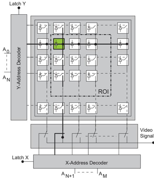
Figure 1 Typical APS detector matrix configuration
