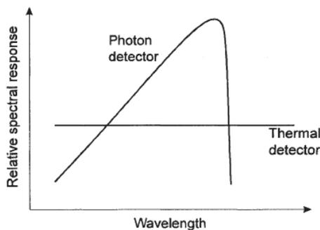
Fig.2. MCT versus microbolometer spectral response
