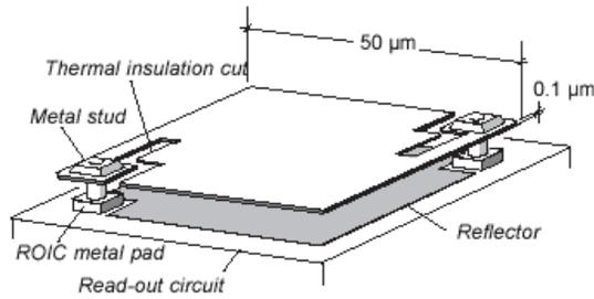
Figure 1: Schematic of microbolometer pixel
