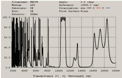
Fig. 4. Typical multi layer filter response
