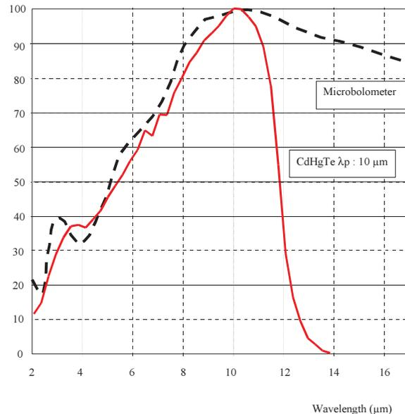
Fig.3. MCT versus microbolometer spectral response. (Courtesy of Ulis)
