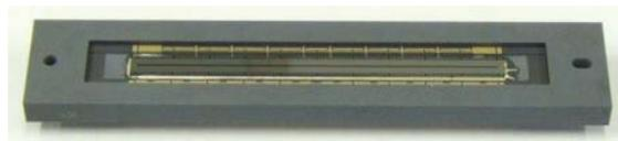
Fig. 5. The packaged CCD
