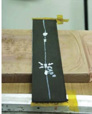
Fig. 6. Picture of a composite sample containing the capillary based sensor design of Fig. 2.
