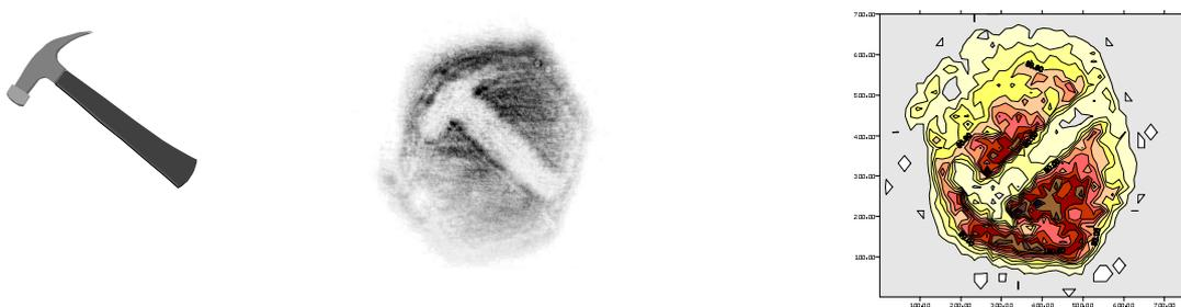
Fig. 3. Example of optical addressing of liquid crystalline panel placed into one arm of Mach-Zehnder interferometer. From left to right are shown: object image superimposed onto 514.5 nm expanded laser beam, phase contrast due to interference of image bearing beam 632.8 nm with reference beam of interferometer and a phase map. The phase difference seen in this case was  $2\pi$  and the phase nonuniformity exceeded  $\pi/4$  mostly due to panel misalignment.
