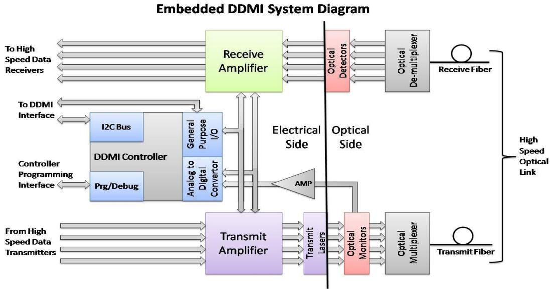
Fig. 6. DDMI system block diagram illustrating the various component of the transceiver module.
