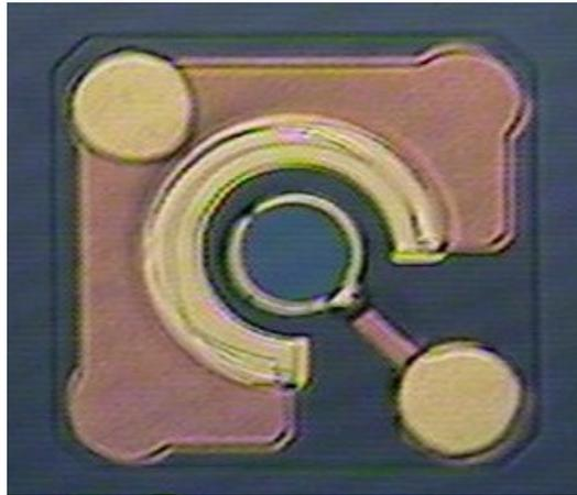
Fig. 3. PIN photodiode fabricated at OptiComp Corp. that can be bonded to an optical bench for a vertical submount in the receiver module.
