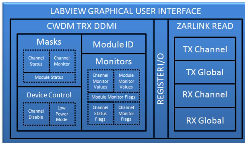
Fig. 7. LabView user interface architecture used for module development.
