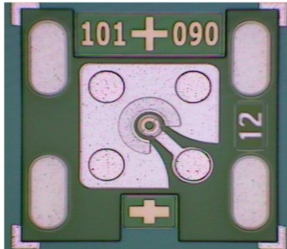
Fig. 1. VCSEL die fabricated on a GaAs wafer in OptiComp Corp. manufacturing facility. This device will be bonded to an optical mounting bench in the transceiver module.
