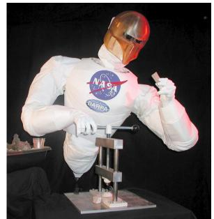
**Figure 4:** The Robonaut is remotely controlled to perform physical tasks by mirroring the actions of a human for potential future NASA missions. Courtesy of NASA Johnson Space Center.
