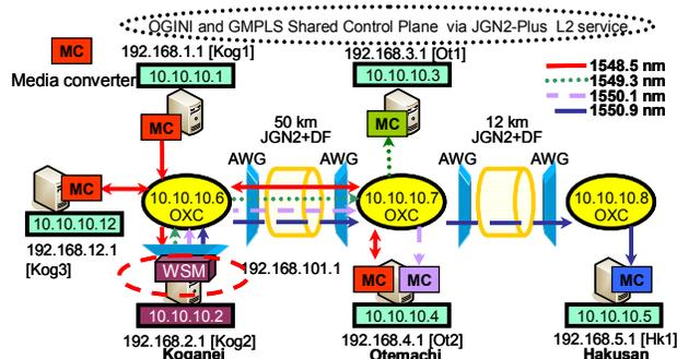
Figure 8. OGINI prototype built on WSON testbed.
