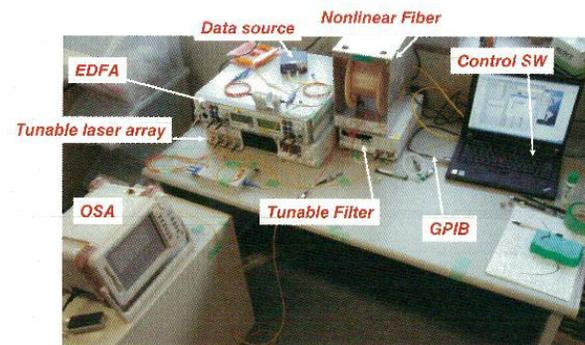
Figure 9. Experimental setup of the WSM.
