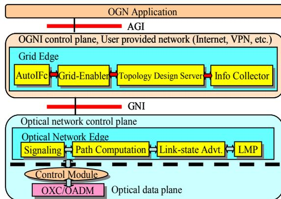
Figure 2. Edge node architecture in OGNI design.
