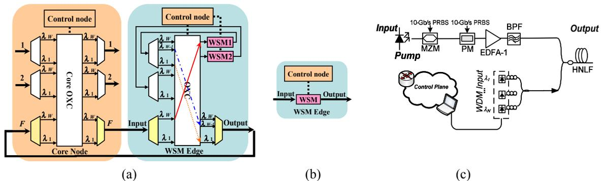
Figure 5. Edge-mode implementation of INS. (a) WSM edge; (b) a lightweight WSM edge; (c) structure of the WSM unit.
