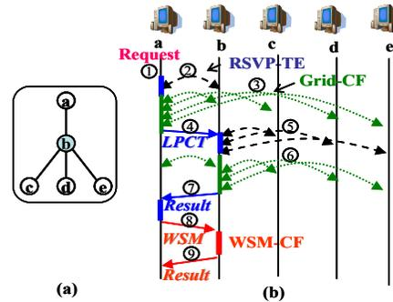
Figure 7. A tree construction example: (a) a specified tree, (b) protocol.
