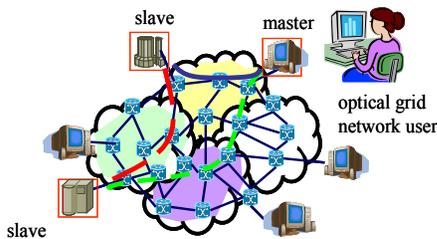
Figure 1. On-demand OGN construction over multi-domain WSONs.
