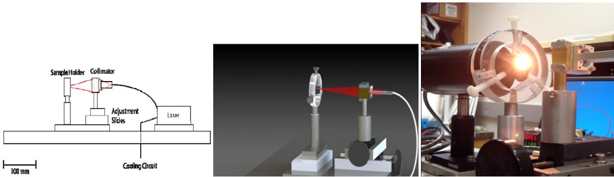
**Figure 13 - Left:** Cross section diagram showing laser (which is 19 individual fiber fed lasers) and the re-collimating optics. **Middle:** Rendering showing beam expansion and imaging as well as sample holder. **Right:** Laser firing at a target (basalt in this case).
