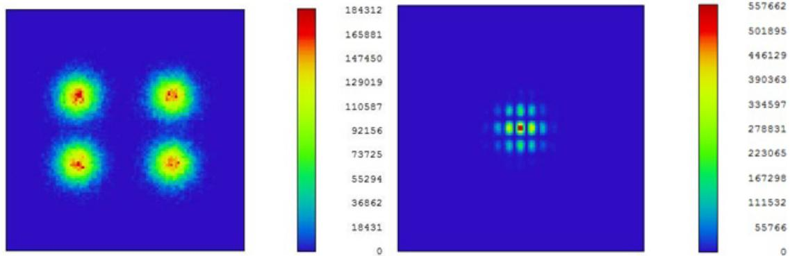
**Figure 3** - Coherent beam combining of a 2x2 laser array in Zemax. The 4 individual elements are shown on the left and then when combined the central peak is intensified and the sidelobes suppressed. With additional elements the peak will grow and the sidelobes will decrease. Our baseline uses a filled close packed array to minimize sidelobes and to maximize the central peak.
