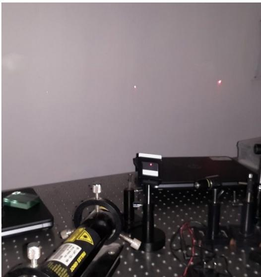
Diffraction of laser through diffraction grating.
