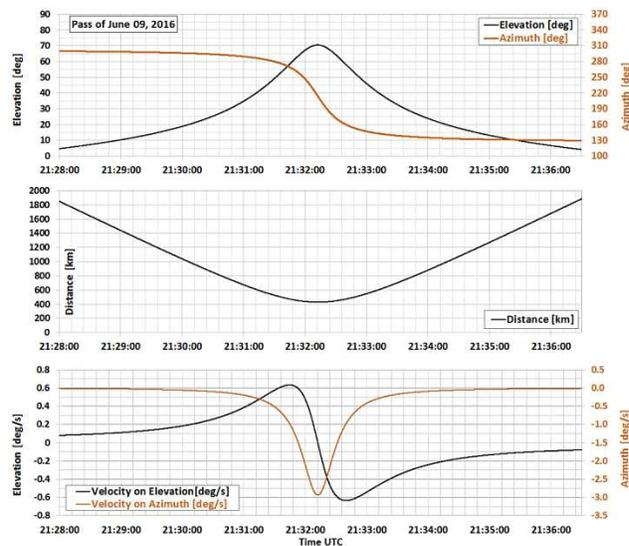
**Fig. 9.** Orbit information of ISS pass for auto tracking test, predicted table is sent by NASA. Maximal velocity is 3.0 deg/sec on azimuth and 0.65 deg/sec on elevation
