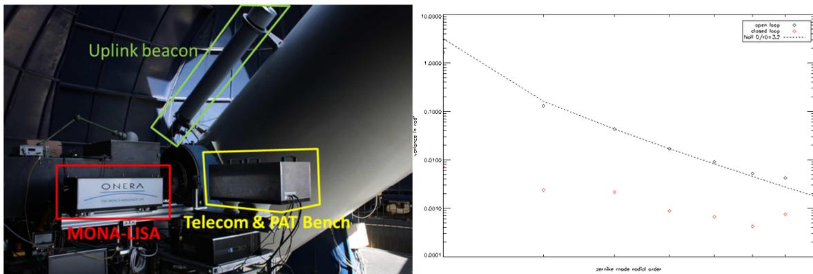
**Fig. 6.** MOLA-LISA AO Bench at nasmyth table [left]. Wavefront variance per Zernike polynomial radial order in open loop (black square) and in closed loop (red square) measured on a star [right]
