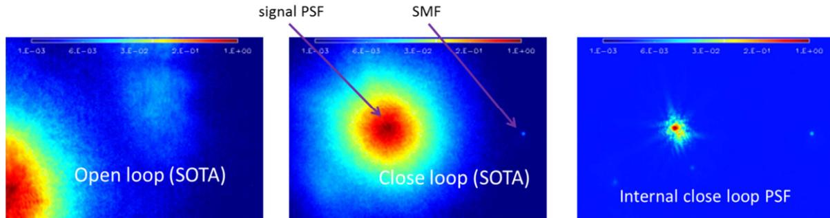
**Fig. 3.** Imaging camera: SOTA signal PSF in open loop (left), SOTA signal PSF in closed loop and SMF (center), internal source used for calibration PSF and SMF (right)
