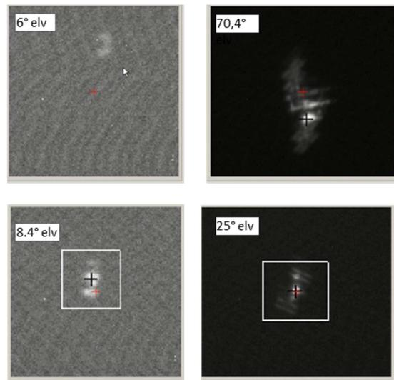
**Fig. 10.** Image of ISS in camera field, auto tracking non-activated (up left) & active (down left), at 25° elevation (down right), and at culmination – 70.4° elevation (up right).
