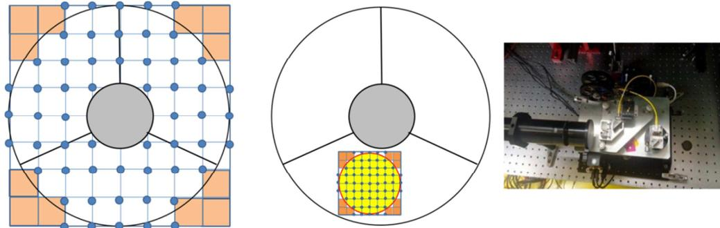
**Fig. 5.** Schematic of the DM actuator grid (dots), located at the angles of SH-WFS subaperture grid (squares). The useful aperture, with telescope spider and central occultation are delimited in black. A  $8 \times 8$  subaperture grid is used on SH-WFS, valid subapertures are whitened [left picture]; DM actuator grid when used on the 40cm pupil taken in the useful aperture of the 1.54m telescope corresponding to the new set-up [middle picture]; CESAR SMF injection module [right picture]
