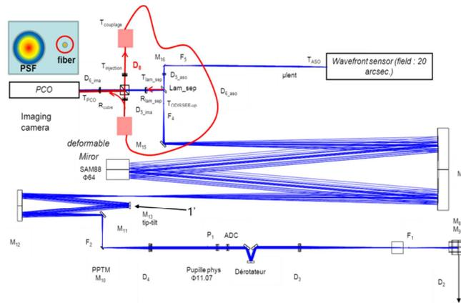
**Fig. 4.** Set-up used for fiber injection experiment using ODISSEE AO Bench
