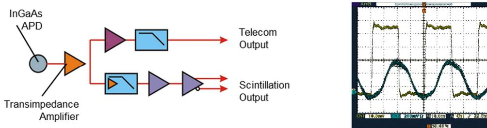
**Fig. 7.** [left]: Monopixel Detector used for both telecom detection and scintillation measurement; [right]:Temporal response of the detector modified for OPALS:green Optical 50 MHz square signal (reference), blue : APD response
