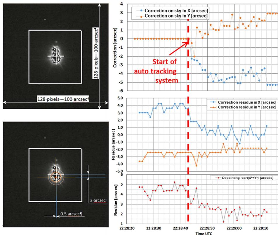
**Fig. 8.** [left] Image of the laser beam from SOTA on the Hammamatsu tracking camera with auto tracking system activated; [right] corrections and residual error using auto tracking for the 22<sup>nd</sup> of June 2015 pass
