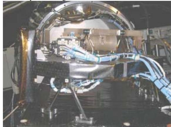
Figure 6 : Optical bench assembly in front of vacuum chamber.
