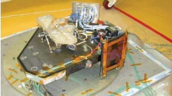
**Figure 7: Optical Bench Assembly during mechanical tests.**
