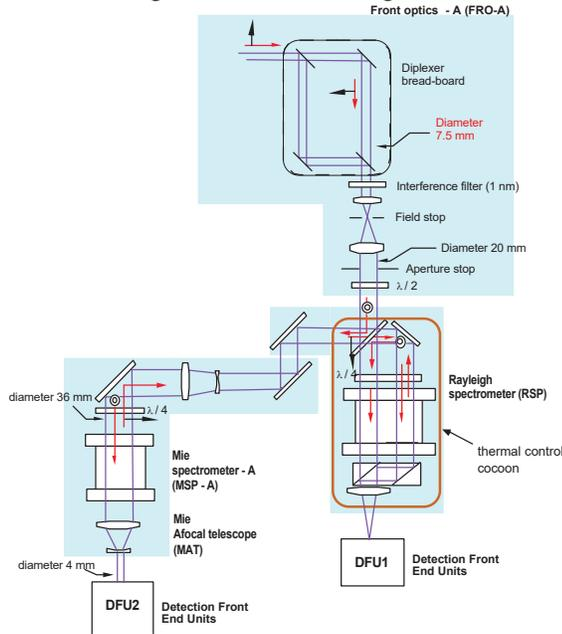
Figure 5 : PDM principle sketch.
