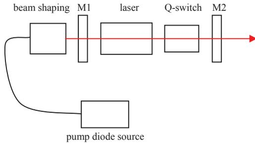
Fig. 2: Laser setup longitudinally pumped from one side with up to 300 mJ pump energy in 300  $\mu$ s pulses at 1 kW peak pump power
