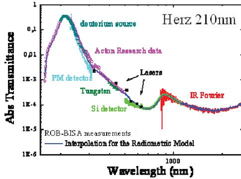
Fig. 7: Herzberg filter transmission combining CSL, BISA-ROB measurements and compared to ARC data and extrapolated radiometric model.
