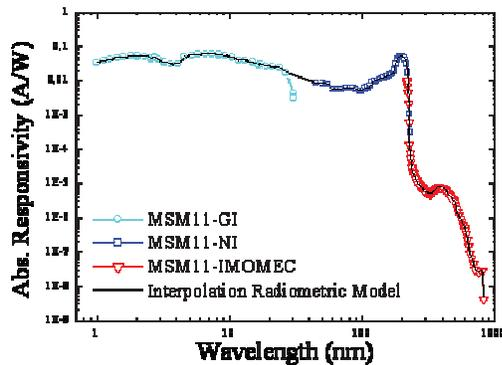
Fig. 4: MSM11 detector responsivity combining PTB (Gi and NI) and IMOMECE measurements.
