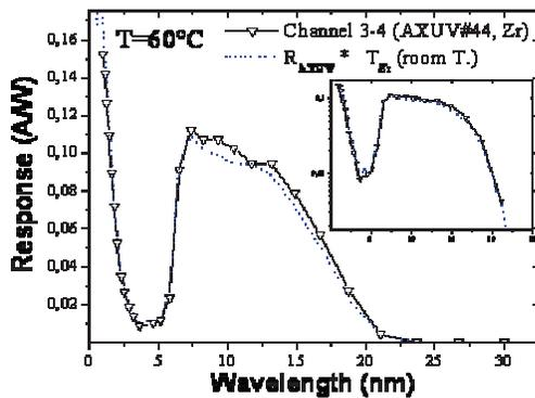
Fig. 8: Absolute spectral responsivity (in A/W) of the Zirconium filter channel between 1 nm and 30 nm. For comparison, the dotted line represents the model used in the LYRA radiometric model (detector  $R \times$  Filter T).
