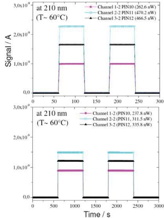
Fig. 9: Absolute signal (in A) of the Herzberg channels as a function of time at 210 nm for a short period (top) and for a long period (bottom).
