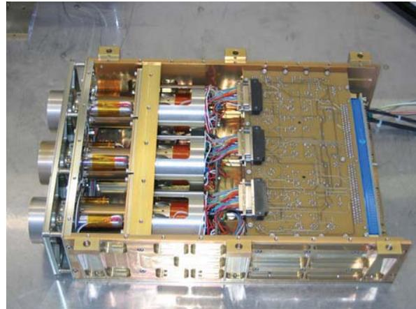
Fig. 1: View of the 3 heads in the FM, each with 4 channels are aligned behind an aperture door
