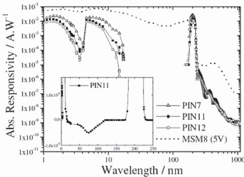
Fig. 5: Typical absolute spectral responsivities (A/W) measured for PiN and MSM diamond detectors.
