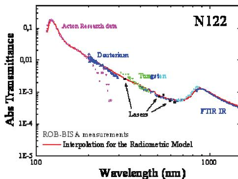
Fig. 3: Measured transmission and radiometric extrapolation for the N122 filter
