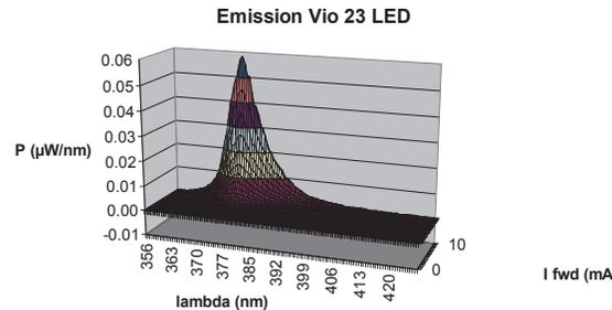
Fig. 6: 380 nm LED emission spectra versus forward current
