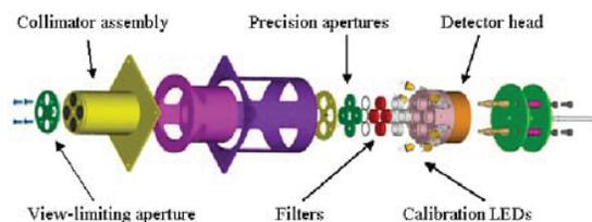
Fig. 2: Exploded view of one of the three identical LYRA units. Each unit contains 4 spectral channels. The collimator, the filters, the LEDs and the head can be seen. The detectors are hidden by the head. The incoming radiation is coming from the left side
