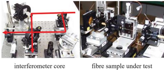
Fig. 7: Mach Zehnder test interferometer operating at 10.6 μm used to estimate the suppression of higher order modes.
