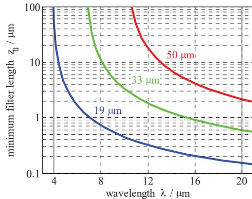
Fig. 1: Required single-mode fibre length to safely remove all cladding modes. The calculation assumes a silver halide step-index fibre of numerical aperture  $NA=0.15$ . Three different core diameters are shown.
