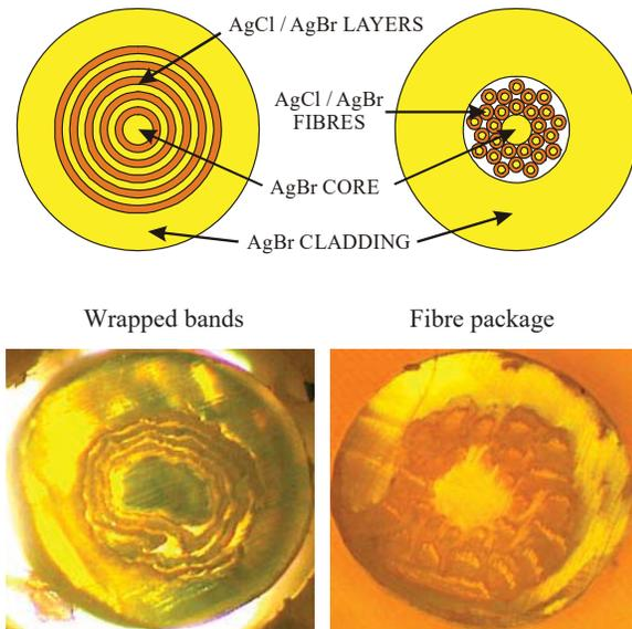
Fig. 6: Second set of realised photonic crystal fibres.
