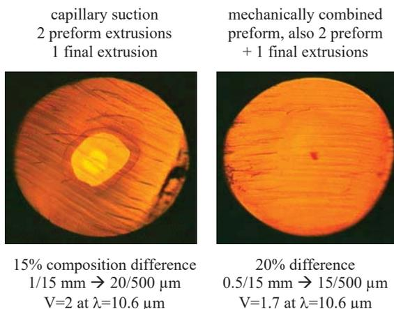
Fig. 4: Realised silver halide fibres, both single mode.
