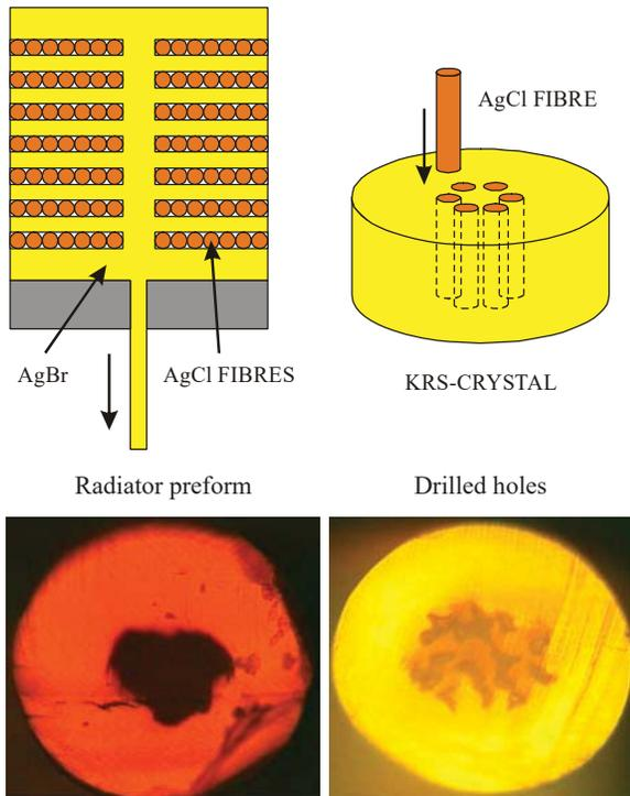
Fig. 5: First set of realised photonic crystal fibres.
