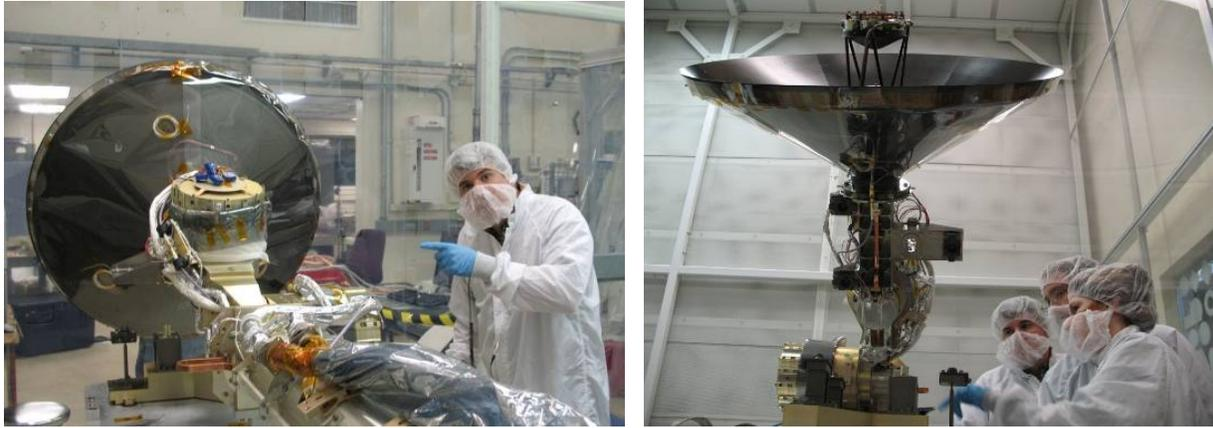
Fig. 13. a) The team investigates - the full motion of the High Gain Antenna comes close to the optical cable routing configuration. b) Richard Chuska motions that the High Gain Antenna is now fully integrated to the gimbals and boom arm.
