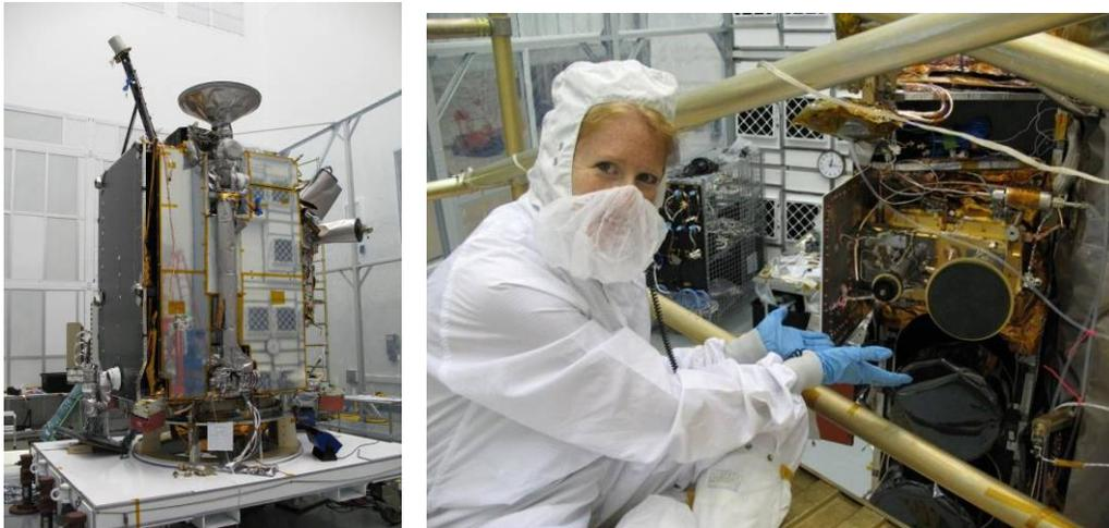
Fig. 16. a) LRO fully integrated with the LRT and LOLA systems, b) Melanie Ott pointing out the location of LOLA on LRO
