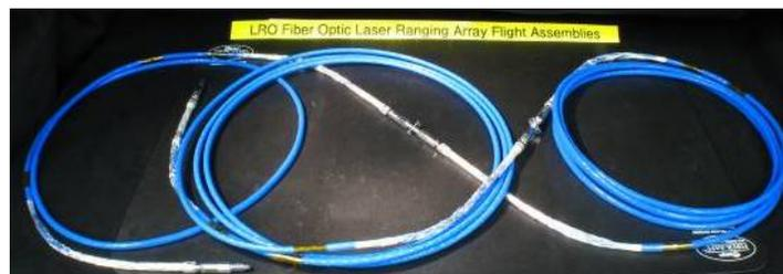
Fig. 10. Flight Array Bundle Assembly Set
