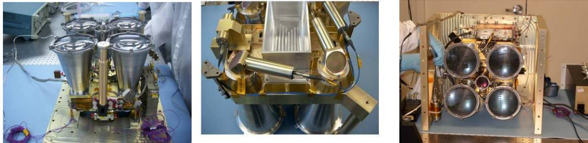
Fig. 1. The Mercury Laser Altimeter consisted of four telescopes with fiber coupled from each to four individual detectors.[6]
