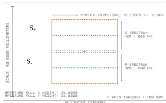
Fig. 3: Footprint diagram at detector indicating both  $S_+$  and  $S_-$  polarisations in the spectral direction. In the spatial direction a  $16^\circ$  swath is imaged 15 times. For each of the 15<sup>th</sup> viewing directions three field points are indicated: one on-axis and two at the edges of the field ( $\pm 8^\circ$ ).
