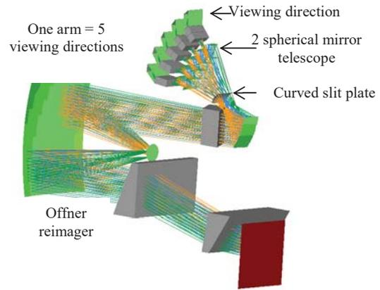
Fig. 5: 3D view of a wide field SPEX2Earth optical concept for SWIR wavelength range, showing the light coming through a set of five viewing directions being combined at the slit and reimaged onto one of the sixth detector parts by an Offner system. Five viewing directions form one arm.
