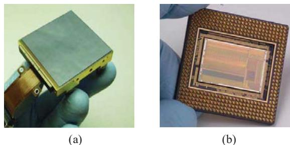
Fig. 4: (a) Teledyne H2RG detector; (b) Teledyne SIDECAR ASIC
