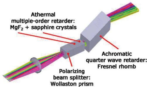
Fig. 1: Optical configuration for the polarization encoding system.
