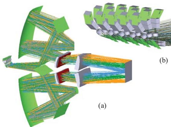
Fig. 2: 3D view of (a) 16 degrees FOV SPEX optical concept for ISS; (b) zoom on the entrance optics showing 15 viewing directions each consisting of polarization optics, telescope, folding mirror and field lens with a double slit.
