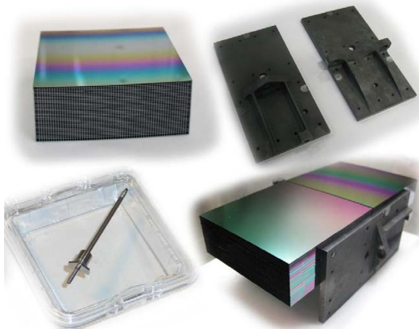
**Fig. 3.** Photos of the components of a SPO mirror module. From top left to bottom right: A SPO stack with 45 plates; a CeSiC® bracket pair; one of the three dowel pins; an assembled mirror module (without pins).
