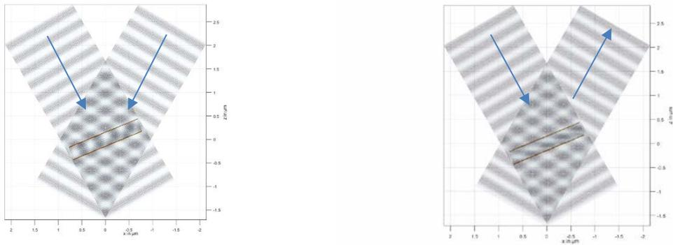
Fig. 2: Left side: the interference pattern resulting from a symmetric holographic exposure setup, right side: interference pattern resulting from the opposing wave approach
