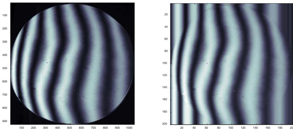
Fig. 5: left side: a typical Moiré-pattern generated by a test setup for an Offner-grating in an even interference field, right side: extended pattern to achieve a square matrix that is beneficial for the numerical processing – the numbers on the x- and y- axes indicate pixel numbers
