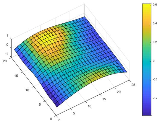
Fig. 6: Moiré lines transferred into a surface figure of a corresponding wave front, by this method an optical designer is able to predict the performance of a spectrometer system – the information about the wave aberration is coded in the distance and curvature of the fringes – the examples shows a PV-value for the wave aberration of about 0.8 periods (note the edges have to be neglected)
