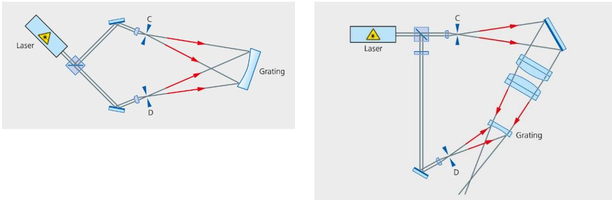
Fig. 1: The principle holographic setup approaches are shown. Left side: the symmetric holographic exposure setup, right side: in relation to the substrate surface the waves are primarily counter propagating
