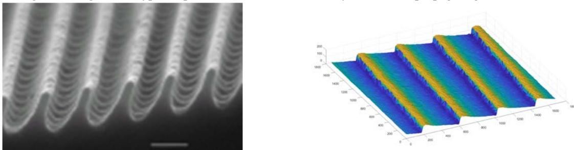
Fig. 4: Left side: deep developed photoresist grating SEM picture with a nearly symmetric profile (tilted symmetric exposure), right side: photoresist grating AFM picture (opposing wave approach)
