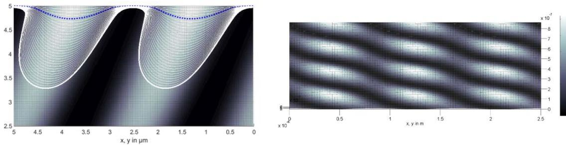
Fig. 3: Left side: photoresist grating simulation with a nearly symmetric profile due to holographic exposure setup in Fig. 1 left, right side: typical spatial modulation of solubility for counter propagating waves
