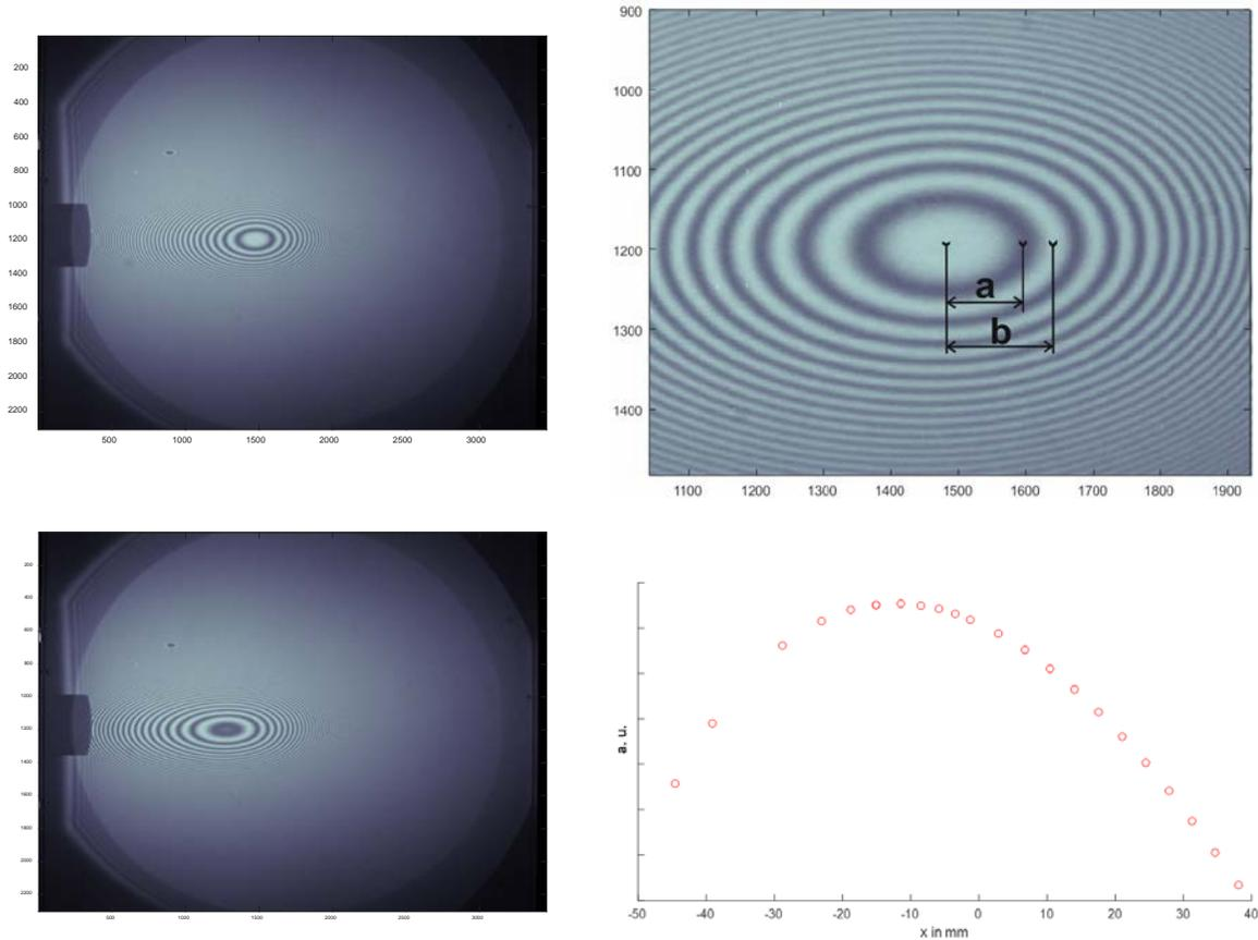
Fig. 7: a) Moiré-pattern of the whole clear aperture of the VLS grating (circular, diameter 100 mm);
