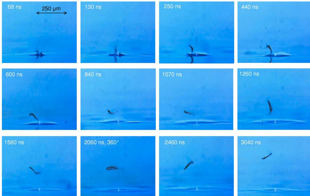
**Fig. 5** Dynamics of a dry PEN foil specimen with 100  $\mu\text{m}$  diam that is catapulted from a glass slide. The specimen was first completely dissected and then catapulted by a 20- $\mu\text{J}$  pulse focused through a 20 $\times$  objective, NA=0.5, onto the rim of the specimen. The plasma luminescence indicates the location of the laser focus. The specimen performs one revolution within 2  $\mu\text{s}$ , corresponding to an initial rotation frequency of 500,000 rps.
