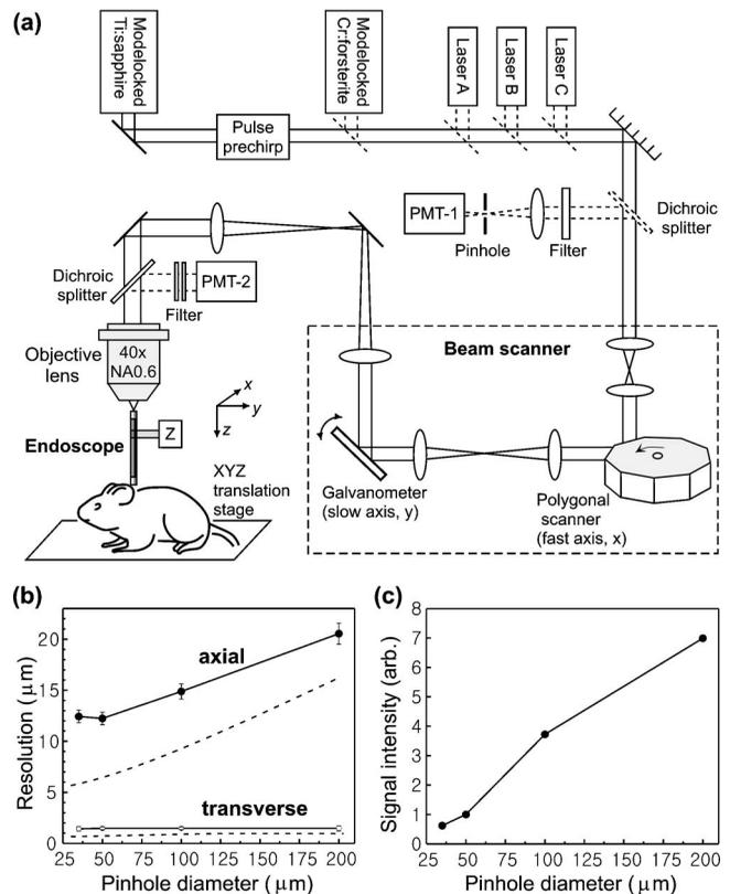
**Fig. 1** (a) Schematic of the microendoscope imaging system and (b) spatial resolution and (c) signal strength in confocal microendoscopy measured with different pinhole sizes. Dotted lines in (b) represent theoretical diffraction-limited resolution of a 0.45-NA objective lens.
