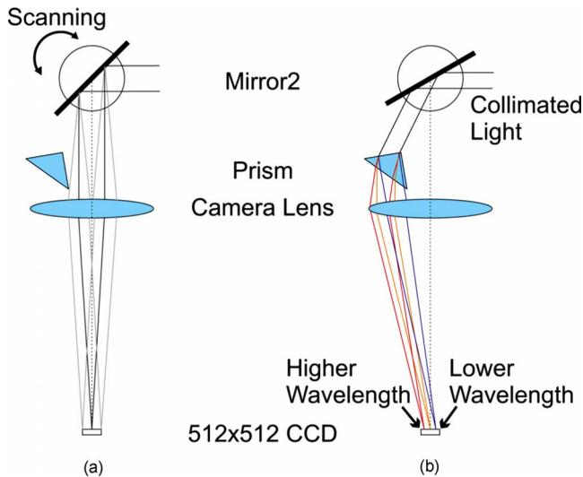
**Fig. 3** Grayscale (a) and multispectral (b) beam paths. Shorter wavelengths exit the prism with the largest deviation angle. Dispersed light is focused on the CCD camera. The position on the detector is directly related to wavelength. Mirror 2 is stationary in the multispectral mode of operation.
