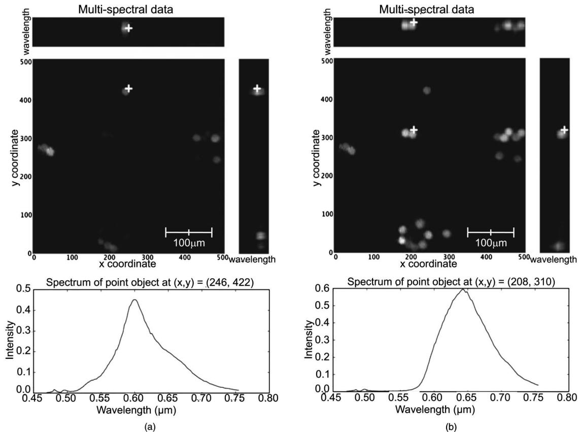
**Fig. 7** Fluorescence images from 15- $\mu\text{m}$  microspheres at wavelength (a) 578 nm and (b) 639 nm, and spectra associated with image point indicated by the white cross.
