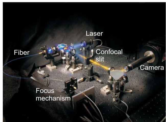
**Fig. 2** Photograph of the confocal microendoscope.
