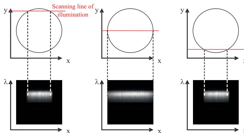
**Fig. 4** Relationship between spatial location (top graphs) and spectral frames (bottom graphs). The lines in the upper images represent the slit illumination profile as it scans across the y-axis of the field of view. The lower images show the dispersion introduced by the prism at the selected scanning positions.
