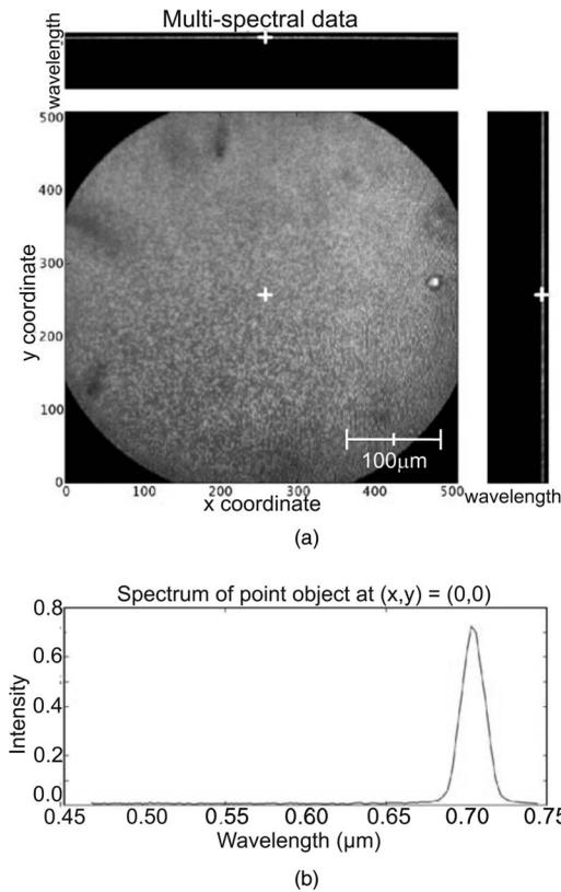
**Fig. 5** Image of the illuminated fiber bundle using a lamp with a 700-nm optical filter. (a) Cross-section planes of the data cube and (b) spectrum of the image point indicated by a white cross. The intensity is unitless because it is scaled relatively to the maximum intensity in the image.
