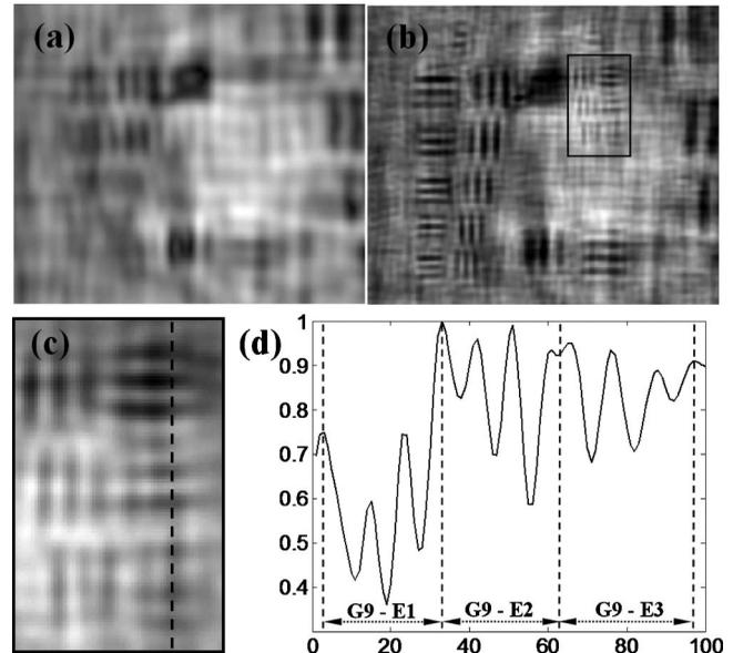
**Fig. 3** Experimental results for VCSEL point source illumination case: (a) reconstructed image using conventional DIHM, (b) reconstructed image using SR DIHM approach, (c) magnified area corresponding with the rectangle in (b), and (d) normalized cross section along the dashed line in (c).
