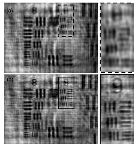
**Fig. 4** Experimental results for violet laser point source and USAF test: (a) reconstructed image using conventional DIHM and (b) reconstructed image using SR DIHM approach.
