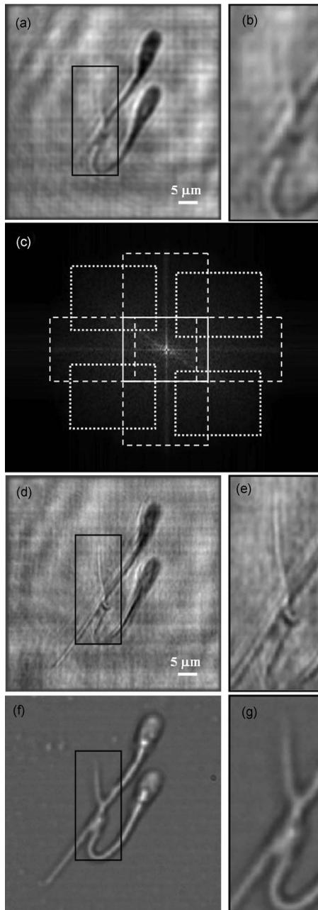
**Fig. 5** Experimental results for violet laser point source and sperm cells biosample: (a) reconstructed image using conventional DIHM, (c) generated SA from the addition of eight off-axis elementary apertures, (d) reconstructed image using SR DIHM approach, and (f) reference image (0.8 NA objective lens) under spatially coherent broadband illumination. Images in (b), (e), and (g) are magnified areas of the black rectangles included in (a), (d), and (f), respectively.
