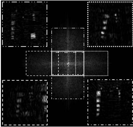
**Fig. 2** Generated SA in the VCSEL point source illumination case coming from the addition of four off-axis elementary apertures. At the corners are the four bandpass images used in the SA generation.
