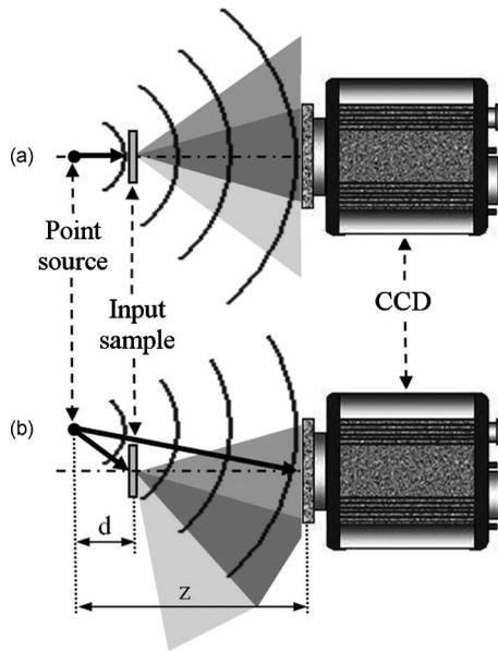
**Fig. 1** Sketch of the SR DIHM setup: (a) on-axis and (b) off-axis illumination cases.
