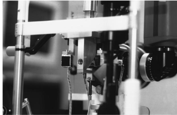
**Fig. 1** OLCR pachometer mounted on a clinical slit lamp (Haag Streit, Switzerland). The LCD and the fixation laser signal are placed in front of the front lens of the slit lamp, allowing the observer to direct the instrument with biomicroscopic stereopsis. The pilot lasers are attached horizontally and converge on the focal distance of the slit lamp, facilitating the alignment of the instrument with the x-y-z control of the slit lamp.
