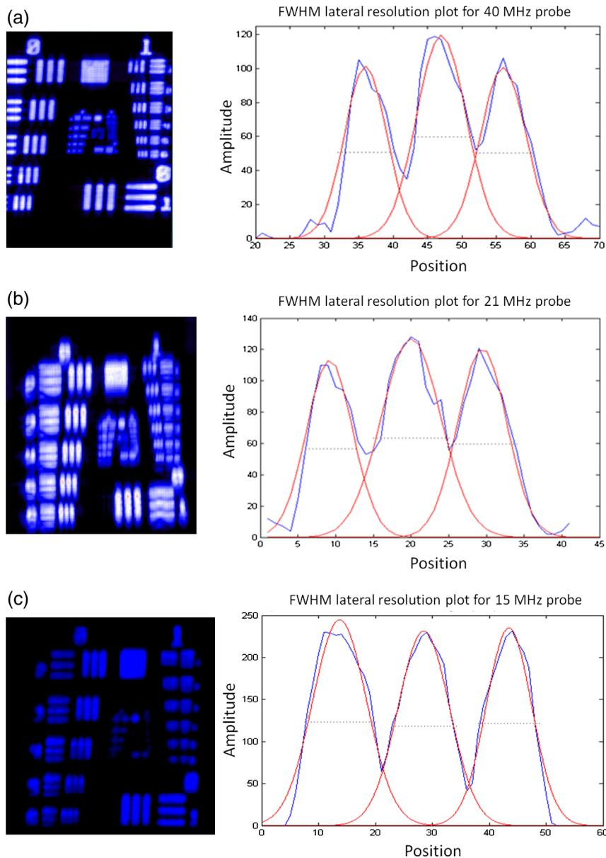
**Fig. 2** The maximum intensity projection (MIP) images of the 1951 USAF target scanned by (a) 40 MHz, (b) 21 MHz, and (c) 15 MHz frequency transducer probes along with the intensity profiles and the fitted Gaussian functions.
