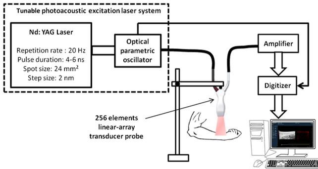
**Fig. 1** Schematic of the experimental setup used in this study. Combined photoacoustic (PA) and high-frequency ultrasound (US) imaging within human forearm skin using linear-array transducer probe.
