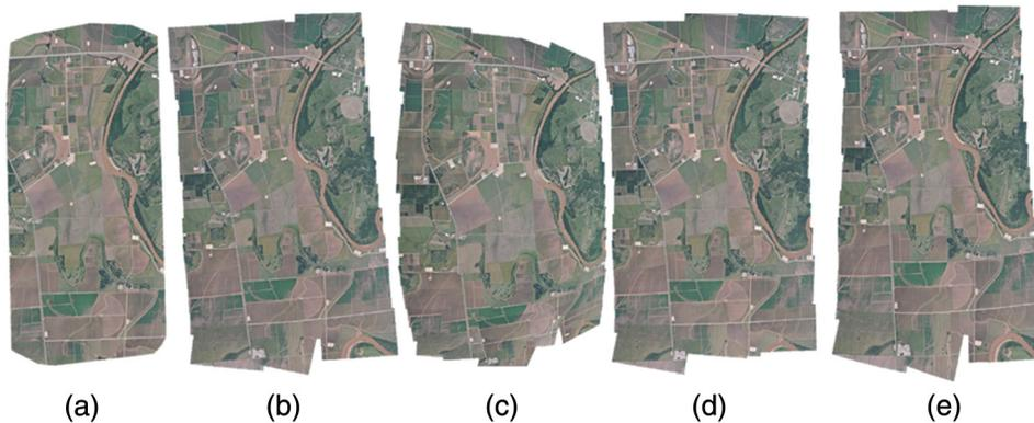
**Fig. 2** Mosaicked images from 70 images captured in six flight lines within the green box shown in Fig. 1 (site 1) using (a) Pix4Dmapper, (b) Autostitch, (c) Photoshop-auto, (d) Photoshop-spherical, and (e) Photoshop-cylindrical.
