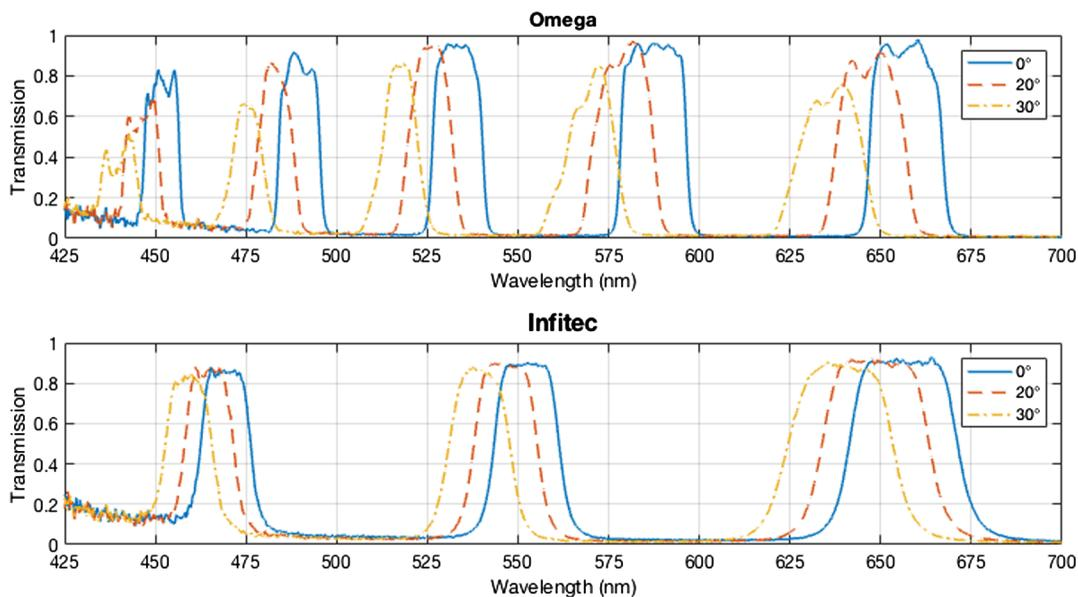
**Fig. 6** Drift as a function of viewing angle measured on Omega filters and Infitec filters.
