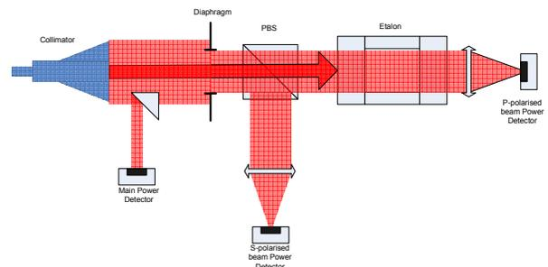
Fig. 2: Setup of transmission measurement
