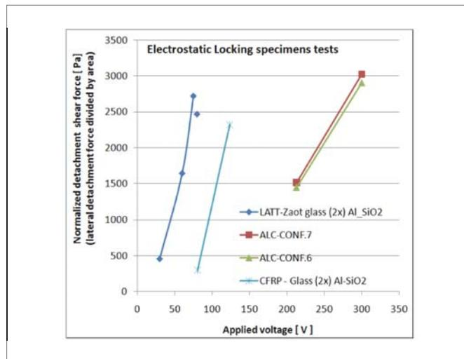
Fig. 3. Pz values at different applied voltage required Pz pressure can be achieved by using a voltage of about 120-150 V (cyan line).
