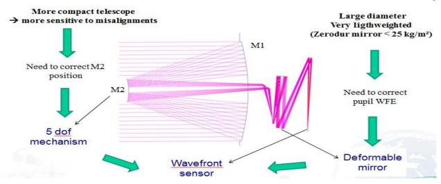
Figure 5. Implementation of active optics proposed in the frame of TANGO project for the next generation of space telescope for Earth observation
