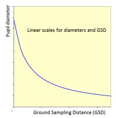
Figure 1. Entrance pupil evolution with respect to the ground sampling distance for a given orbit and for a given MTF performance. Improvement in GSD can affect significantly the entrance pupil size.
