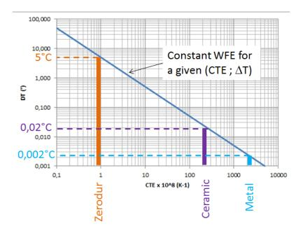
Figure 4. Trade-off for primary mirror material selection. For a given acceptable WFE degradation, different amplitude on thermal gradients can be accepted. Due to thermal orbital fluctuations, the higher is the acceptable thermal gradient the lower is the correction loop frequency.
