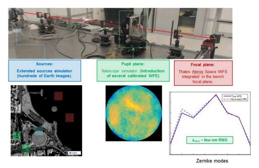
Figure 10. WFS validated on a dedicated bench able to simulate hundreds of Earth images, to simulate tens of telescope WFE. The results show a very good phase retrieval accuracy around few nanometers.
