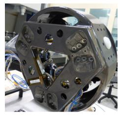
Figure 9. Five DoF mechanism with its 6 actuators and its optimized Si3N4 structure
