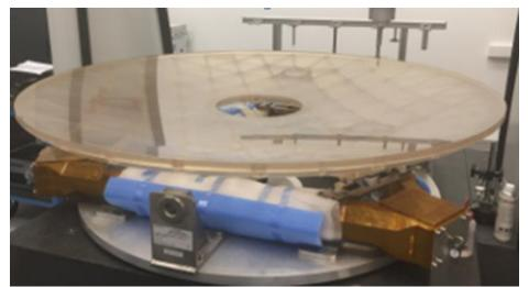
Figure 7. M1 Mirror on instrument Si3N4 main frame. This 1,5 m Zerodur mirror has a total mass around 25 Kg/m<sup>2</sup>.
