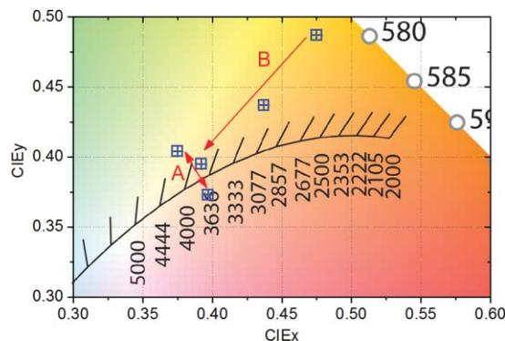
**Fig. 4** Change in color coordinates if the red to green doped area is changed (arrow A) and if the TMM004 to TCTA ratio is varied at the phosphorescent to fluorescent emission layer interface (arrow B).
