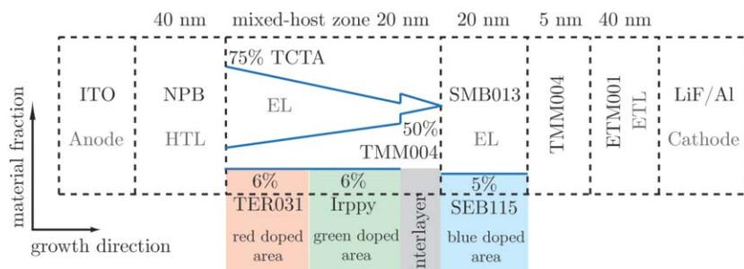
**Fig. 1** Hybrid white OLED stack with a phosphorescent red and green mixed-host emission layer zone and a fluorescent blue emission layer separated by an exciton blocking interlayer.
