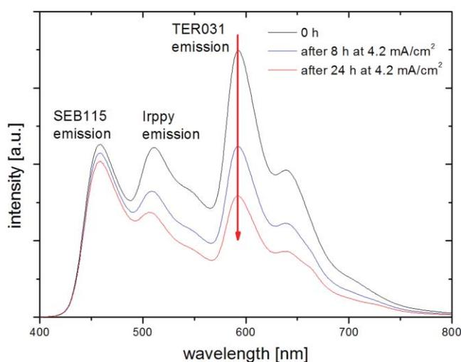
**Fig. 6** OLED spectra taken at 0, 8 and 24 h after device stressing with 4.2 mA/cm<sup>2</sup> (initial 1000 cd/m<sup>2</sup>).
