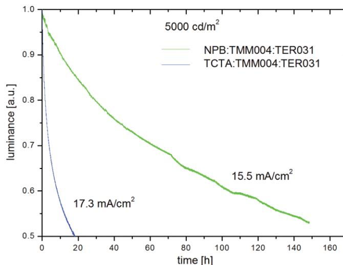
**Fig. 7** Luminance of different monochrome TER031 red OLED versus time of stressing at 5000 cd/m<sup>2</sup>.
