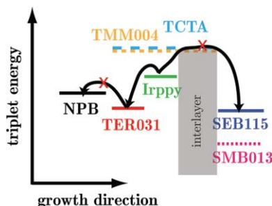
**Fig. 3** Triplet energy levels of the employed organic materials and possible triplet exciton diffusion paths.
