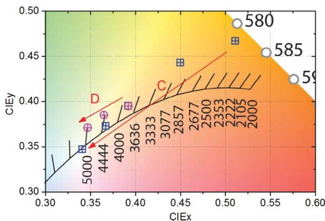
**Fig. 5** Change in color coordinates if the electron-blocking layer thickness is increased (arrow C) and if the blue emission layer thickness is decreased (arrow D).
