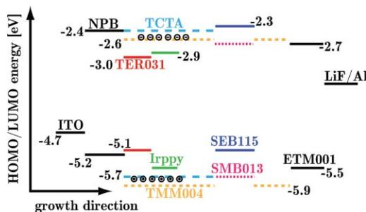
**Fig. 2** HOMO and LUMO energies of the employed organic materials with TCTA as hole and TMM004 as electron conductor.
