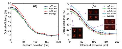
**Fig. 6** Optical efficiencies after adding Gaussian noises with zero mean and standard deviations from 0 to 200 nm to the height distributions of the (a) 1-D and (b) 2-D phase masks. They are calculated at the designated exposure planes and take the average (black lines). Insets of (b): simulated light intensity distributions at four planes separated by 0.3 mm with low noise of  $\delta = 5$  nm (left), medium noise of  $\delta = 40$  nm (middle), and high noise of  $\delta = 100$  nm (right).
