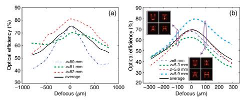
**Fig. 7** Optical efficiencies at various defocus locations of the (a) 1-D and (b) 2-D phase masks. They are calculated at different exposure planes and take the average (black lines). Insets of (b): simulated light intensity distributions at four planes separated by 0.3 mm at  $-100 \mu$ m defocus (left) and  $+100 \mu$ m defocus (right).
