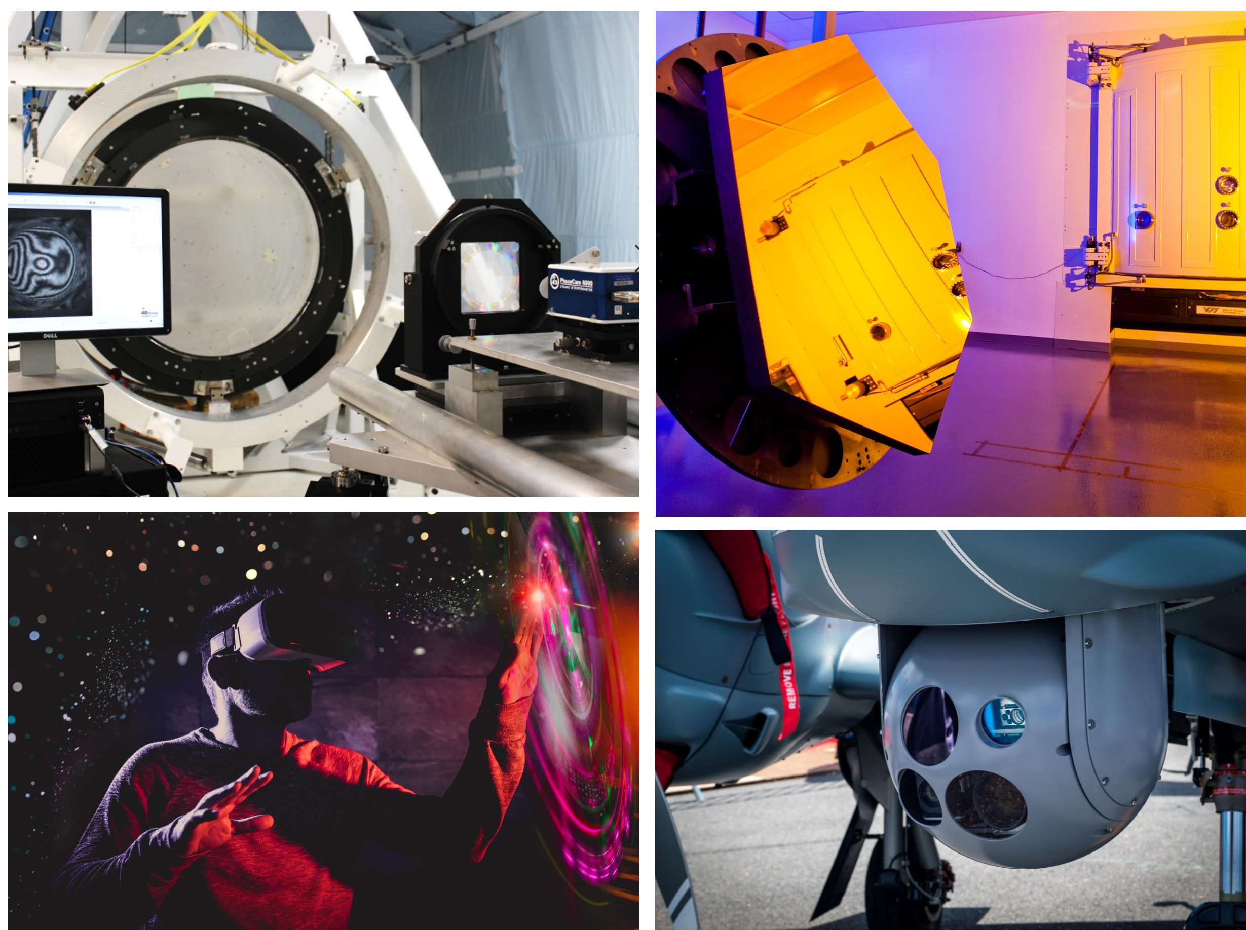
Fig. 2 CGHs are used for surface measurement, alignment, and final verification of a wide variety of optical components and systems. Applications include the world's largest lenses for the Rubin Observatory (LSST) (top left), the primary mirror segments for the James Webb Space Telescope (top right), high-volume complex lenses for next-generation AR/VR headsets (bottom left), and freeform mirrors needed for high performance systems that fit within tight mechanical constraints (bottom right).
